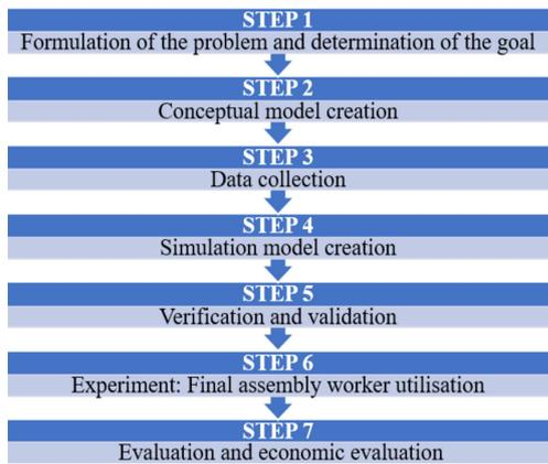
Fig. 1. Seven steps of simulation project for assembly line (source: authors).
