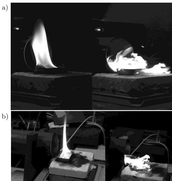
Fig. 4. Extinction of the diesel fuel flame (a) and gasoline flame (b).
