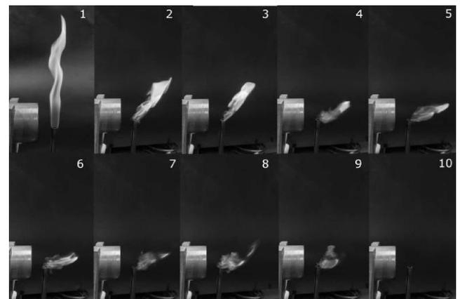
Fig. 5. Extinction of the natural gas flame.
