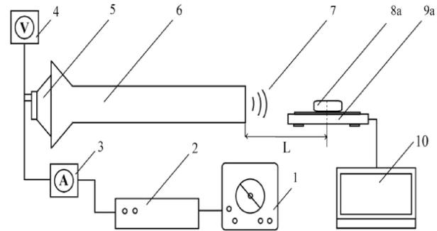
Fig. 1. Scheme of the experimental setup for the liquid fuels extinction [4].
