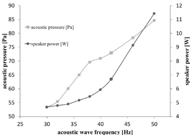
Fig. 6. Speaker extinction power and acoustic pressure as a function of acoustic wave frequency.
