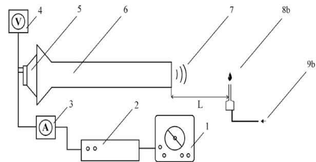
Fig. 2. Scheme of the experimental setup for the natural gas extinction [4].
