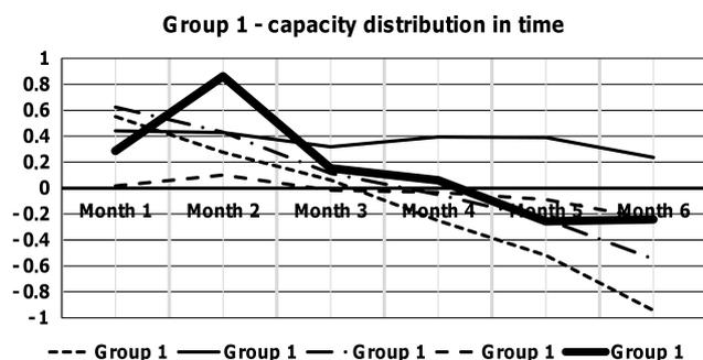
Fig. 3. The distribution of shifts which results from the difference between the production capacity and order load on individual machines in group 1. The bold line illustrates the course of the overall production capacity of this group.
