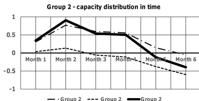
Fig. 4. The distribution of shifts which results from the difference between the production capacity and order load on individual machines in group 2. The bold line illustrates the course of overall process of production capacity of the group.
